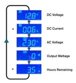
DC Voltage Input voltage available from the battery supply.
