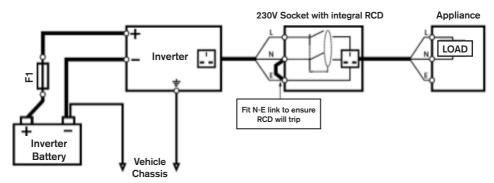
Fig3 - Example RCD installation
