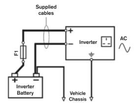
Fig1 - Example single battery system
